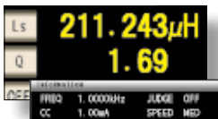
L, Q 표시화면 (1 kHz, Constant Current 1 mA 측정)
